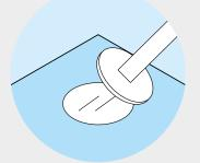
With the metal discs in position, carefully lower the poles at a 45 degree angle towards the disc. Snap in place with the disc and magnet central to each other.
